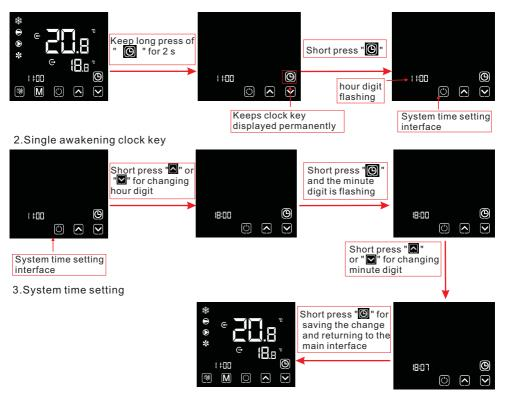
Notes: After the permanent awakening of clock key, if it is not cancelled by user, the main interface will display the clock key permanently. Under the clock setting interface, if short press " " , the change will not be saved and return to the main interface; if there is no operation for 20s, the system will automatically memorize user's setting, and return to the main interface.
