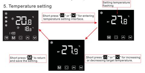
Notes: Under the temperature setting interface, if short press " ", the system will return to the main interface without any changes saved; If there is no operation for 5 s, the system will automatically memorize users setting, and return to the main interface.
